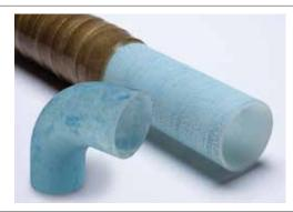
The PVDF HV-Liner from AGRU is an economical alternative to traditional fabric backed pipes. The surface-treated PVDF pipe has a three-dimensional surface structure which provides an optimal bonding to the FRP structure. The piping systems are available in PVDF, PVDF-FLEX, and PVDF-el ESD. The pipes can be produced in diameters from 20 – 400 mm.
