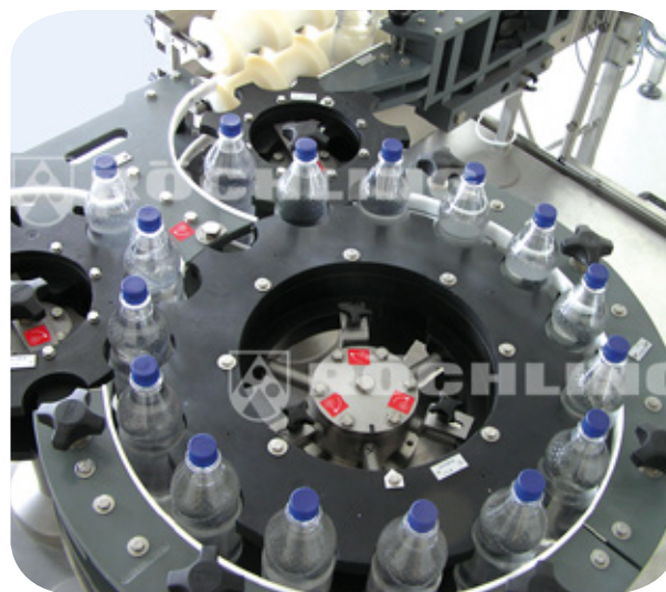
Star wheels and guides machined from Polystone® M Black (UHMW-PE)
