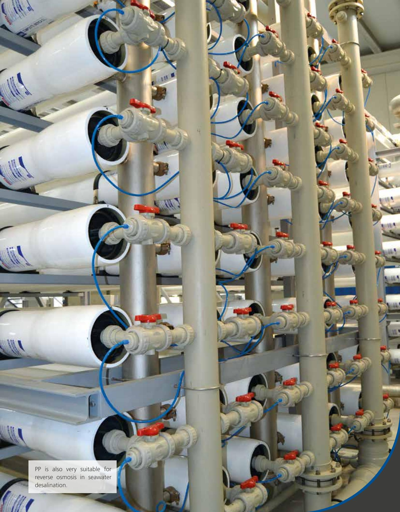
PP is also very suitable for reverse osmosis in seawater desalination.
