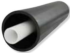
**Double containment piping systems** are prefabricated as standard and can be connected using simultaneous butt welding, after spacers have been welded in, or using cascade welding.
